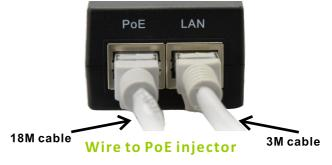
4. Connect Ethernet cable from the camera into the port marked 'PoE'. 5. Connect the 3M cable into the 'LAN' port and the other end on your router.
